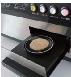
Reflection measurement method for solids
